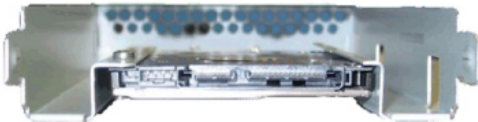
Figure 7.18: Hard Drive/SSD Installed in Driver Carrier
