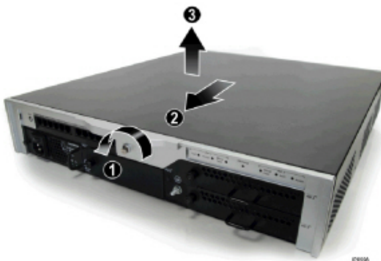
Figure 4.6: MXe III/MXe III-L/MXe III Server - Removing the Cover
