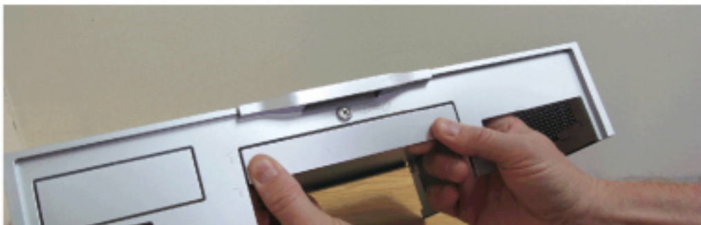
Figure 7.11: Removing Blanking Panel
