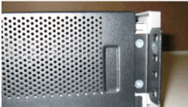
Figure 4.11: CX II/CXi II Controller Rack-Mount Installation - Attaching Brackets to Controller
