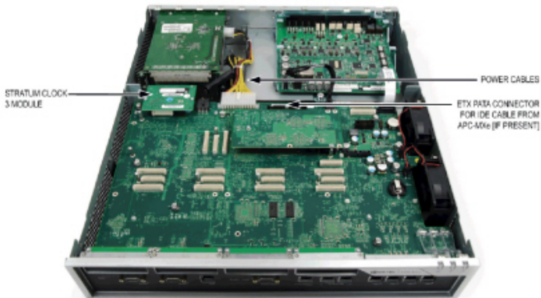
Figure 7.3: Removing the Power Cable
