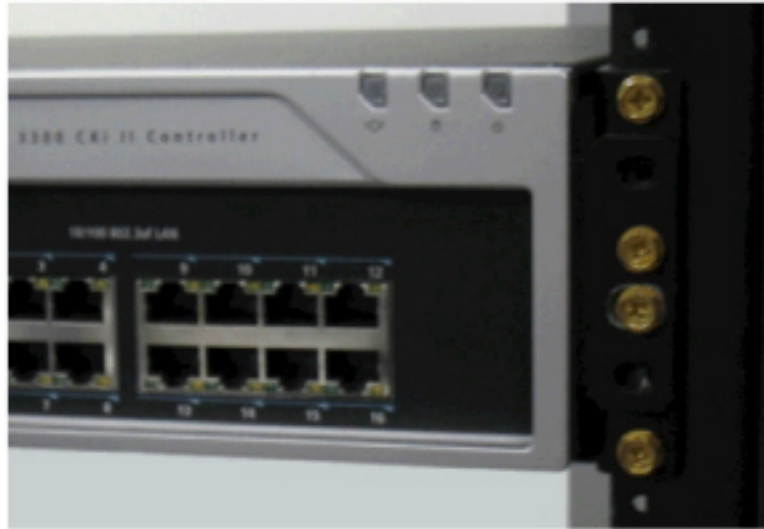
Figure 4.12: CX II/CXi II Controller Rack-Mount Installation - Fastening Angle Brackets to Rack Frame
