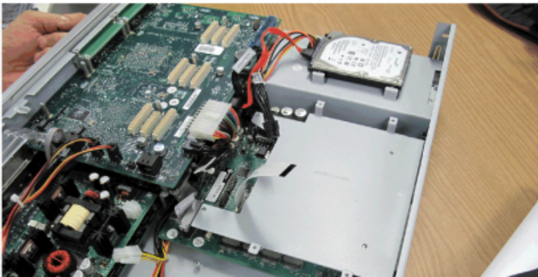
Figure 7.14: AOB Mounting Plate in Position
