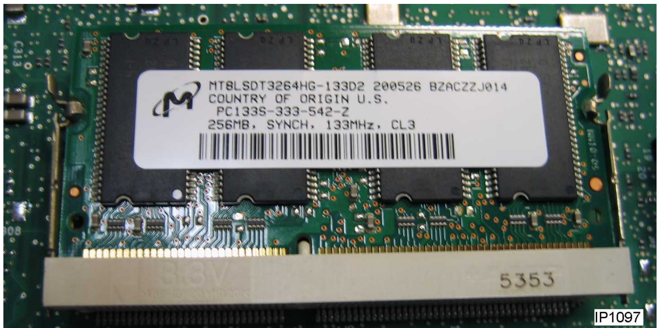
Figure 7.28: Memory Module - AX, MxIII
